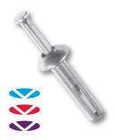
Used with Versico's Termination Bar or Seam Fastening Plates to secure membrane to concrete block, brick, or structural concrete walls. A zinc-plated steel pin provides excellent corrosion resistance while the zinc alloy body provides excellent holding power.
