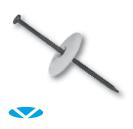
Pre-assembled HPV Fastener and Polymer seam plate applicable to steel, wood and CDX plywood decks. Used to secure VersiGard reinforced membranes.
