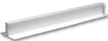
This profile is extruded from the same weather-resistant TPO or PVC compound as the membrane. The Rib Profile is secured to the TPO or PVC roofing membrane to simulate a standing seam metal roofing system. The physical dimensional stability of the profile is enhanced with fiberglass and the rectangular profile provides exceptional shadow lines for aesthetic appeal.
