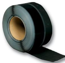
Reinforced Termination Strip (RTS) combines reinforced EPDM with 3"-wide Quick-Applied tape for additional membrane securement. A 9" version with 3"-wide Quick-Applied tape on both sides permits securement of perimeter sheeting on mechanically attached systems.
