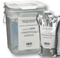
A single-component, moisture-curing, elastomeric polyether sealant that is compatible with Versico's EPDM membranes. It is designed to provide a flexible, durable and long-lasting seal around hard-to-flash penetrations. The sealant's consistency allows for quick pocket filling without mixing. Unused sealant is usable for up to 30 days if pouch is resealed with original cap. Black one-part pourable sealer is black in color.
