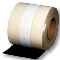
10" RUSS (shown) is used in place of narrow-width sheets to secure membrane in the perimeter of the roof on mechanically attached systems. 6" RUSS is also available and is used to secure membrane at the base of vertical walls for additional membrane securement without penetrating the sheet.
