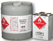
Used to clean both new and in-service VersiGuard EPDM membrane and VersiWeld TPO membrane prior to the welding process. It helps to loosen and remove dirt and other contaminants from the surface of the membranes and leaves a suitable surface for application of adhesive or primer. Please refer to the Technical Data Bulletins for specific instructions for EPDM and TPO applications. Membrane cleaner is clear in color.
