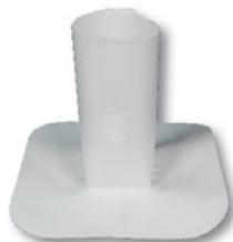
Fabricated using VersiWeld detail membrane and VersiFlex membrane and designed to flash square metal tubing. A split and overlap tab are incorporated into these parts to allow the flashings to be opened and wrapped around a square penetration with an obstruction. Additional sizes and colors available through special order.
