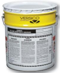
A high-strength, solvent-based contact adhesive that allows quick bonding of cured EPDM membranes to various substrates. Designed for bonding VersiGard (black and white) non-reinforced, VersiGard reinforced, and Epichlorohydrin membranes to approved substrate.
