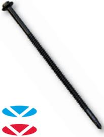
Used with Versico's Metal Retrofit Roofing System to secure membrane and RTS to structural steel purlins. Compatible with 2" Polymer Plates. Provides superior back-out resistance in standard 16-gauge Purlins.
