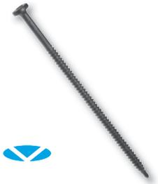
Applicable to steel, 22-gauge and heavier, CDX plywood and wood plank deck types. Can be used to secure VersiGard reinforced membranes, RTS and for insulation securement. Longer fastener sizes available as special order. Not applicable for securing TPO and PVC membranes.
