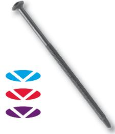
A specially designed fastener with a ½" drill point used for attaching VersiGard, VersiWeld and VersiFlex membranes to structural steel purlins (up to ¾") in standing seam metal roof retrofit applications.
