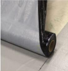
A 40-mil composite consisting of 35 mils of self-adhering rubberized asphalt laminated to a 5-mil woven polypropylene film. Used as an air and vapor barrier/temporary roof, one-piece poly release liner prevents the material from bonding to itself in the roll and is easily removed for installation. May be used as a temporary roof for up to 120 days. Common substrates include concrete, DensDeck®, and SECUROCK®.
