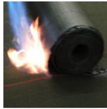
Premium smooth-surfaced SBS torch-applied membranes reinforced with fiberglass mat. Can be used as a base ply in multi-ply systems, as an air and vapor barrier, or as a temporary roof for up to 60 days. Excellent for low temperature applications when use of peel-and-stick membranes may not be possible. Ideal substrates include primed concrete and primed SECUROCK.
