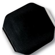
Uncured EPDM laminated to a synthetic rubber adhesive. Used to seal field splice intersections and horizontal-to-vertical transitions of field splices. 12" x 12" T-Joint Covers are available for 30-Year Warranty Systems.
