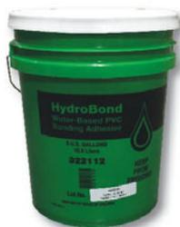
A water-based, wet lay-in, one-sided dispersion adhesive that is used to secure VersiFlex PVC and VersiFleece® PVC membranes to a variety of substrates. Complies with the California Clean Air Act of 1988 (updated in 1997) and California Air Quality Control District's listing of VOC limitations. Meets the requirements of the OTC Model Rule for Single-Ply Roofing Adhesives. Cannot be used with KEE HP, TPO or EPDM smooth-backed membrane.
