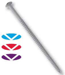
A #14 diameter fastener used for VersiGard reinforced, VersiWeld and VersiFlex membrane securement into structural concrete decks (minimum 3,000psi). Also applicable to insulation securement into steel, wood and concrete decks.
