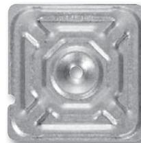
AccuTrac Plates are 3" square flat- or recessed-bottom plates made of Galvalume-coated steel. Used to fasten insulation with the AccuTrac Tool.
