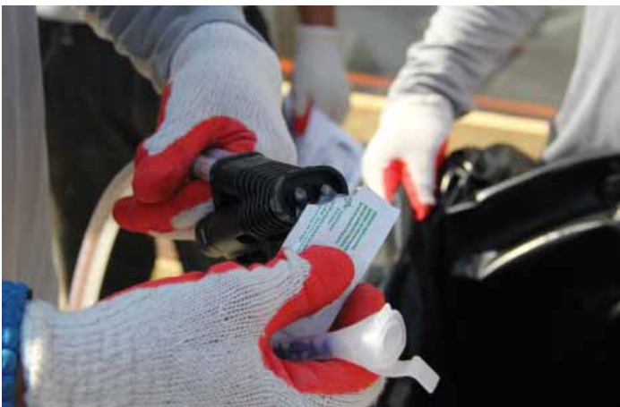
Application of petroleum jelly to spray gun
