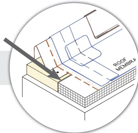
2. When treated lumber is specified, it is recommended that only lumber that has been pressure treated with salt preservatives be utilized. Some lumber preservatives (such as Creosote, Pentachlorophenol, Copper Naphthenate, and Copper 8-quinolinolate) will adversely affect the membrane when in direct contact and are therefore unacceptable.
